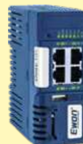
Router for remote maintenance
